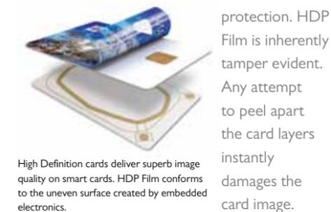
High Definition cards deliver superb image quality on smart cards. HDP Film conforms to the uneven surface created by embedded electronics.
